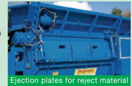
Ejection plates for reject material
