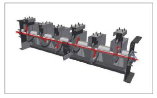
With the new Inline-lubrication-System, time-consuming lubrication processes are a thing of the past. The lubrication is done by the crankshaft axis. Special distributors ensure a reliable and uniform grease supply of each bearing.
